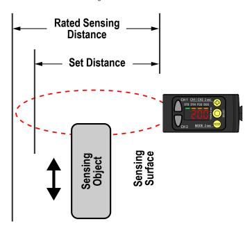
**Hysteresis (Differential Travel)**—With respect to the distance between the standard sensing object and the sensor, the difference between the distance at which the sensor operates and the distance at which the sensor resets.
