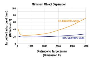
Figure 38. Minimum Object Separation for 5 ms Response Time
